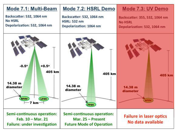
Figure 1. CATS three main Science Modes for operation, with details of each mode's capabilities and operational status.
