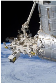
The Japanese Experiment Module - Exposed Facility (JEM-EF) on the International Space Station (ISS). Payloads are robotically attached to the JEM-EF.
